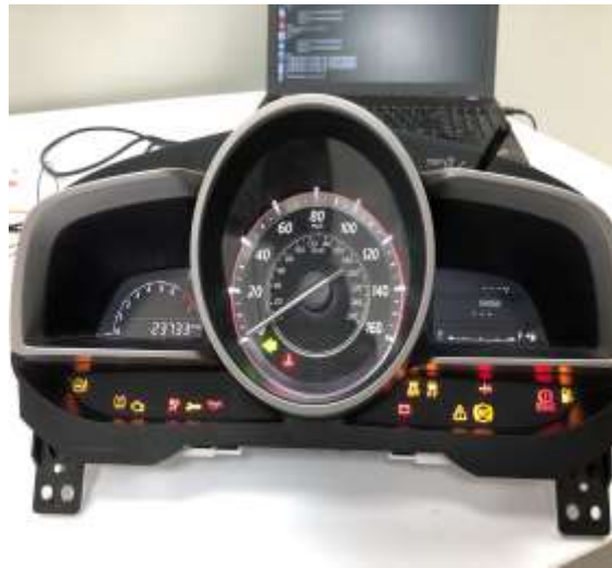
Fig.12. Result of sending right signal CAN frame
