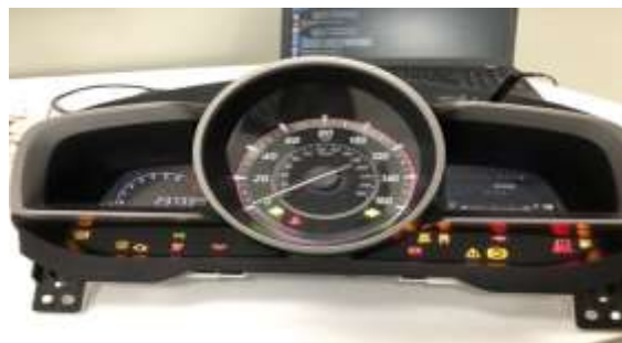
Fig 10. Result of Sending Flasher's CAN Frames
