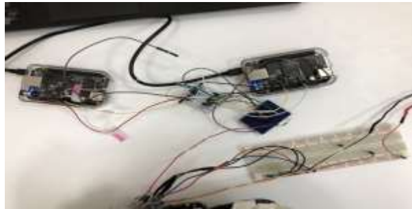
Fig. 8. BBBs, CAN Bus, and Transceivers
