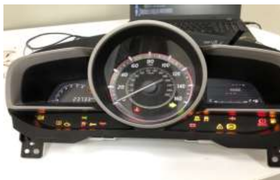
Fig.11. Result of sending right signal CAN frame
